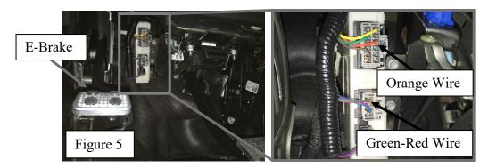
3. Attached 6" wire between Orange wire(Pin 3 on C2498C Connector) and Green-Red wire (On F150) or Red wire (on Super Duty) (Pin 1 on C2498A Connector) using Scotchloks (For F150 supplied Scotchloks can be used, Super Duty are not supplied, recommend using 3M 902). This will activate a continuous +12V to the +12V power pin on the 7pin trailer connector. Refer to Figure 6
