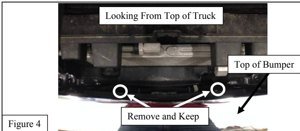
6. If truck has factory hardware in location shown in **Figure 5**, remove the two upper 10mm bolts shown and keep. If it does not have factory hardware move to **Step 7 (If truck has factory hardware, hardware supplied will not be used)**
