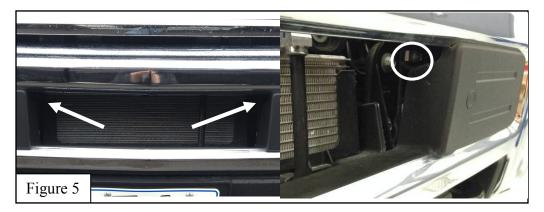
7. Step 7 is only for trucks without factory hardware in locations shown in Figure 5. Slide 1/4"-20 clip nuts over black steel bracket in locations shown in Figure 6 (2 Locations). (Nut side of clip will face toward front of truck)
