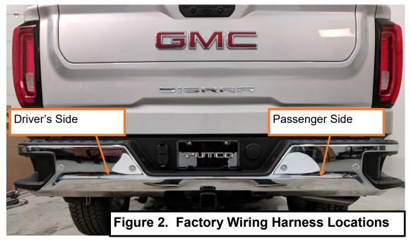
1. Factory wire harness are located behind the rear bumper, near the spare tire, frame rails, and exhaust. Shown in Figures 2 and 3.
