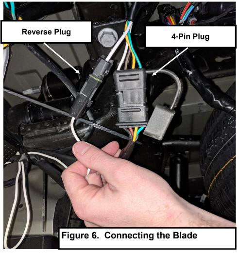
8. With the help of an assistant, test the functionality of the Blade (brake, turn signals, and reverse).
