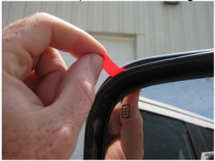
**Step 8:** Now that the mirror cover has been installed, remove the red protective liner from the 3M<sup>™</sup> Tape on the extension arm and install.
