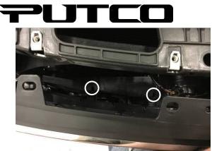
Pull upper grille forward to release upper grille clips. Once out, release 4 bottom metal clips with a flat head screwdriver by pushing down on them through hole in the plastic. Passenger side locations are shown. Repeat on driver side
