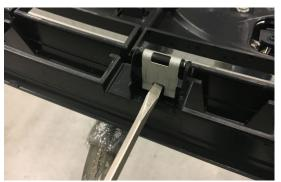
5. Remove grille. <u>Once grille is removed</u>, lay grille on flat surface (Protect grille front face) remove 4 metal clips with screwdriver from bottom of grille and set aside.
