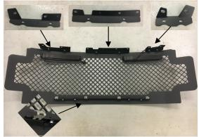
Install all brackets in locations shown. All brackets go on upper side of tabs. Use supplied hardware to mount all brackets. For lower bracket use bracket form step 6 and install so metal clips are facing up.
