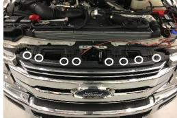
Once cover is removed, remove the top 8 grille screws with 10mm wrench (location shown above)
