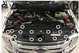
Remove plastic cover by removing 14 retaining clips (number of retaining clips may vary) with flat head screw driver (locations shown above).
