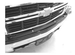
Install bracket with 3/8" bolts and washers. Tighten down with 7/32" hex wrench. Recommend using thread locking compound.
