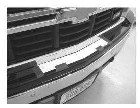
2. Cutout and tape paper template on front bumper. Line front of template up with top lip of bumper.
