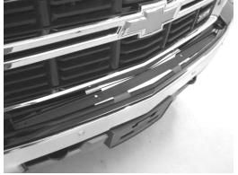
Lay bracket on bumper and line up hole on template with holes on bracket. Verify that bracket is straight on bumper. Once straight, drill two ½" holes (just through plastic) in locations marked on template.
