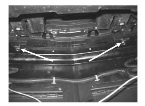
4. Go to back side of bumper. Place two clip-on nuts in holes on steel bumper (Nut facing down in locations shown above).
