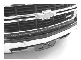
Place 40" curved light bar onto bracket; reinstall hardware as shown in (Figure 1 of Light Installation Instructions). Tighten nut with 7/16" wrench. Route wiring through grill.
