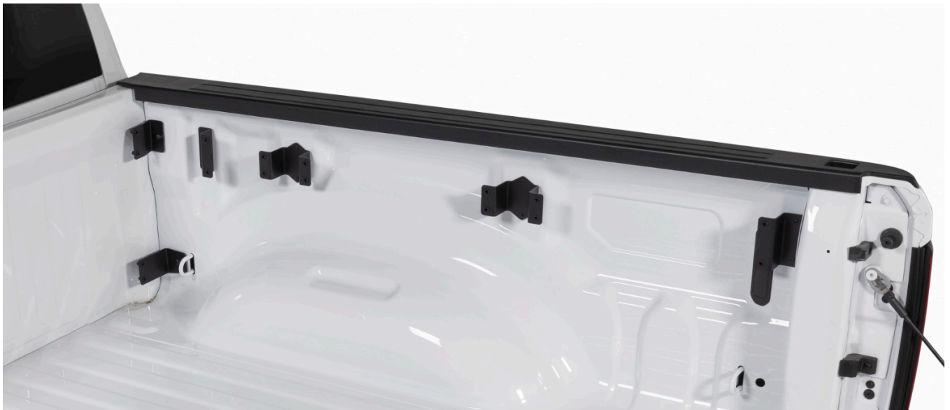
Light Duty Ram with All Brackets Installed
