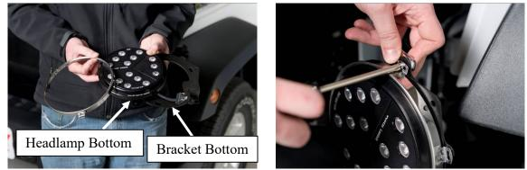
6. <u>Mount New headlamp into bracket</u> using factory retaining ring removed in Step 3 and supplied #6 hardware. Use Phillips screwdriver and 5/16" wrench to tighten. Verify that Putco headlamp is installed with the bottom of the headlamp to the bottom of the bracket. Driver side headlamp is shown above and retaining ring will only mount direction. Putco bracket is the same between Driver and Passenger side.
