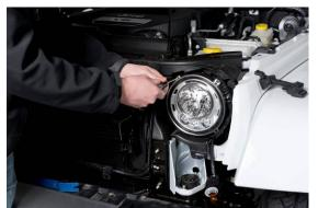
Remove factory light retaining ring by unscrewing (4) T15 Torx screws around perimeter of factory light.
