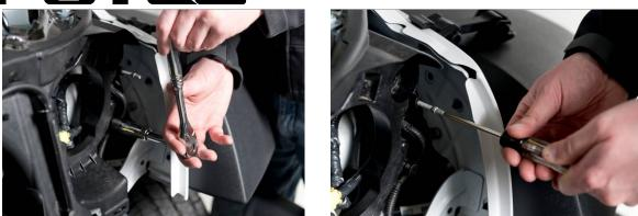
5. Once factory headlamp is removed unscrew the 3 factory mounting pins. The two bottom pins can be removed with a 15mm socket and top can be removed with a T15 Torx bit.
