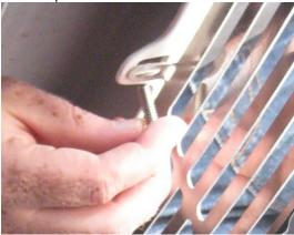
**Step 8:** Secure the Allen Head Bolts with the provided Washers and Nylon Lock Nuts.
