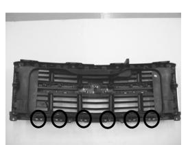
8. Once grille and upper bumper are off the truck. Remove the upper bumper piece from grille. Use a flat head screw driver to unclip the 6 tabs on bottom backside of the grille.
