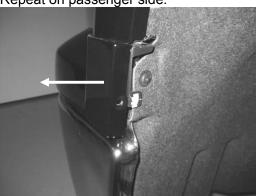
6. Pull out upper bumper end. Driver side is shown. Repeat on passenger side.
