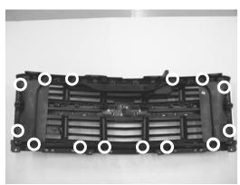
9. Remove shroud from behind grille. Use 7mm wrench to remove 14 bolts.
