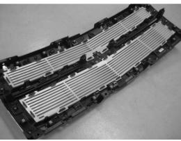
11. Snap in top and bottom Putco grille insert into grille over existing tabs.
