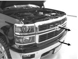
7. Pull grille and upper bumper pieces out away from truck and place face down on scratch free surface. These two pieces will be attached together.
