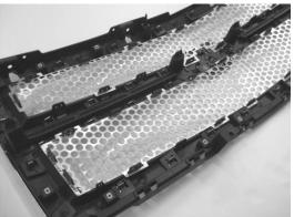
11. Snap in top and bottom Putco grille insert into grille over existing tabs.
