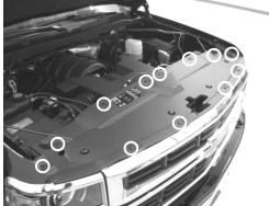
2. Remove plastic cover by removing 12 retaining clips with flat head screw driver (locations shown above).
