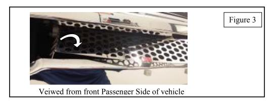
5. Rotate the right leg back up rolling the top edge inside the grille opening. The right leg will then slide through the larger opening for the toe hook as shown in Figure 4.
