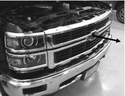
8. Pull grille out away from truck and place face down on scratch free surface.
