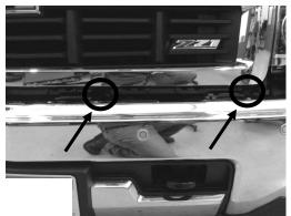
7. Use 10mm wrench to remove total of 4 bolts from bottom of grille. Driver side locations are shown. Repeat on passenger side.
