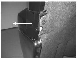
5. Pull out upper bumper end. Driver side is shown. Repeat on passenger side.
