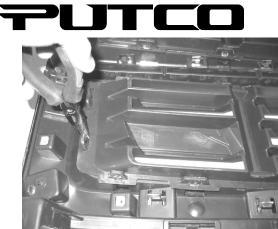
10. Use needle nose pliers to squeeze clip and snap out top and bottom factory grille inserts.
