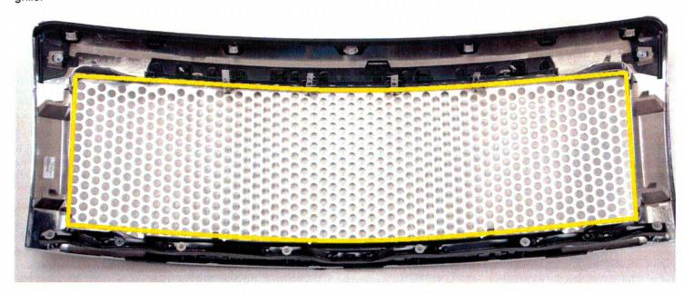
Step 8: After the surround is cut, attach the L brackets with the included washers and nuts. Position the L brackets so it is parallel to the edge of the grille like in the picture shown below.
