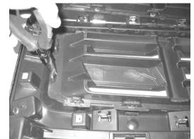
10. Use needle nose pliers to squeeze clip and snap out top and bottom factory grille inserts.
