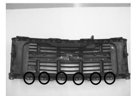
8. Once grille and upper bumper are off the truck. Remove the upper bumper piece from grille. Use a flat head screw driver to unclip the 6 tabs on bottom backside of the grille.
