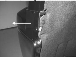
6. Pull out upper bumper end. Driver side is shown. Repeat on passenger side.
