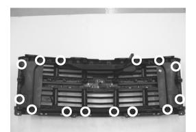
9. Remove shroud from behind grille. Use 7mm wrench to remove 14 bolts.
