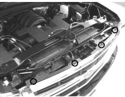
3. Once cover is removed, remove the top 4 grille screws with 10mm wrench (location shown above).
