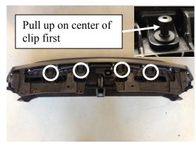
Once factory grille assembly is removed from truck; remove and keep (4) plastic clips on top of grille assembly. Use flat-head screwdriver to pry up center of clip first and pull clip out.
