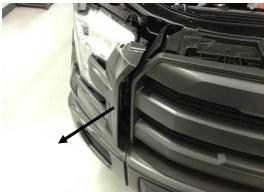
4. Pull out plastic cover around headlight. Passenger side is shown. Repeat on driver side.
