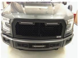
15. Install grille assembly in truck. Once grille is in, snap light covers back in place and close hood. Some adjustment my be required. Reopen hood and unclip light covers. Tighten all hardware, reinstall all factory clips and bolts.
