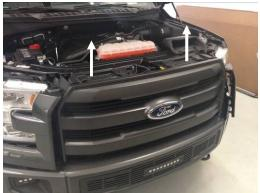
8. Remove factory grille assembly by pulling grille straight up and out.
