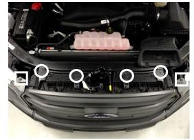
Remove and keep the top (4) grille screws with 10mm wrench (location shown by circles) and (2) plastic tree clips with screwdriver (location shown by squares).
