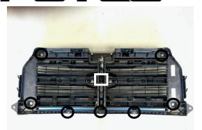
On back side of factory grille assembly, remove (7) 10mm nuts (shown by circles) and (1) 7mm bolt (shown by square). Front side of grille can be set aside, it will not be used.
