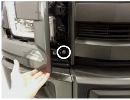
6. Remove and keep (total 2) 8mm bolts securing lower grille to truck. Passenger side location is shown above. Repeat on driver side
