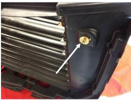
11. If any of factory hardware remains in the back side of the factory grille assembly, remove using a pliers and 10mm wrench. Place back side of factroy grille assembly aside for later installation.
