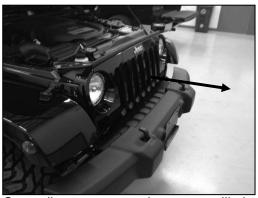
3. Once clips are removed, remove grille by pulling straight out and unhooking the marker lights.
