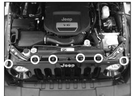
Remove 6 plastic retaining clips with flat head screw driver (locations shown above) by removing center rivet pin first.
