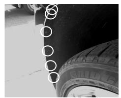
In front driver fender well, remove and set aside (6) 7mm bolts in locations shown. Repeat on passenger side.
