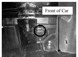
7. Underneath front bumper, use a straight screw driver and unclip (2) plastic clips that hold the grille to the frame. Passenger side is shown repeat on driver side.
