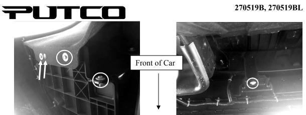
4. Underneath front bumper, remove (8) 10mm bolts and (2) plastic push clips. Locations shown above are of just the driver side locations. Set bolts and push clips aside.
