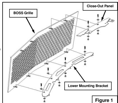
9. Attach the two *Close-Out Panels* to the top of the grille using the supplied hardware. (Passenger Side Shown Fig-1)
