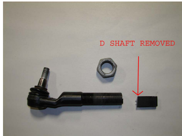
Shaft Trimmed Off
