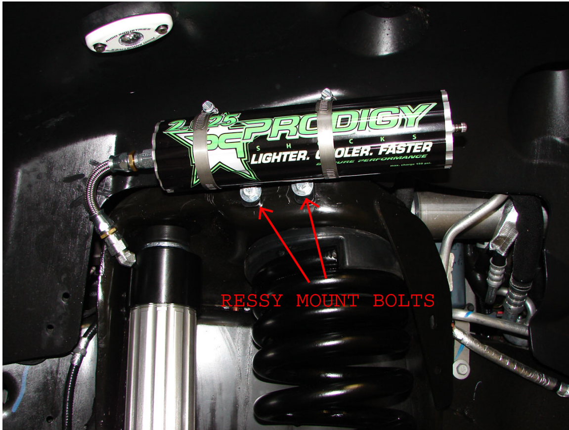
Front Ressy Holder Bolted to the Stock Spring Bucket
