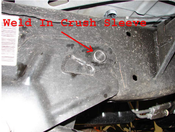
Weld in Crush Sleeve Installed In Frame
