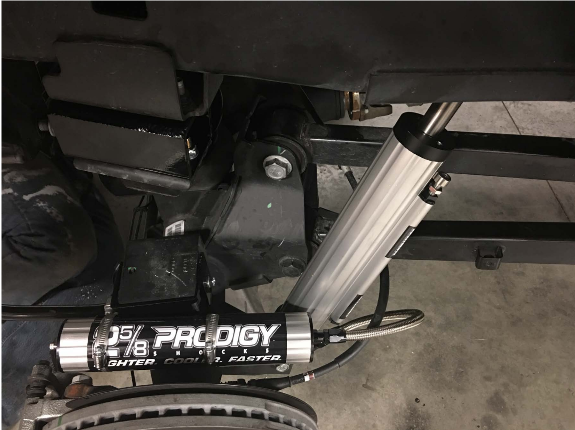
Reservoir Mount Secured to the Bottom Bump Stop Pad
