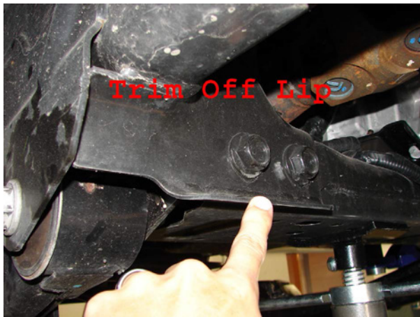
Driver Side and Passenger Side Rear Sheetmetal to Trim
