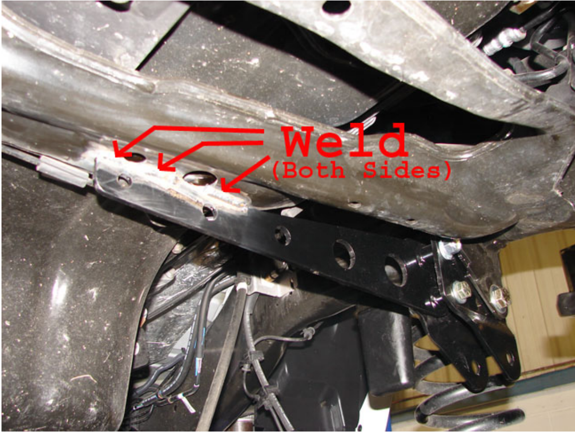
Track Bar Bracket Cross Brace Welded to OEM Cross Member
