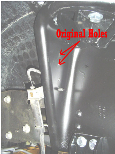
2005 – 2007 Brake Line Relocation
