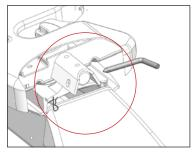
Plate attaching points are covered, limiting visibility to a small "site" hole
