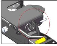
Plate attaching points are visible and accessible for easy removal and re-installation
