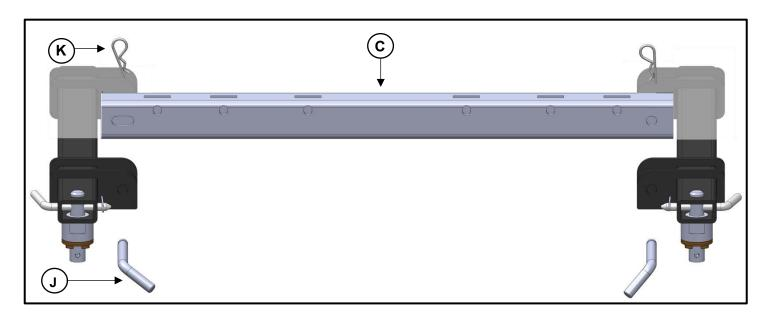
7. Once hitch pins and clips are secured, set your fifth wheel in the corresponding mounting locations and secure with 1/2" hitch pins (not included).
