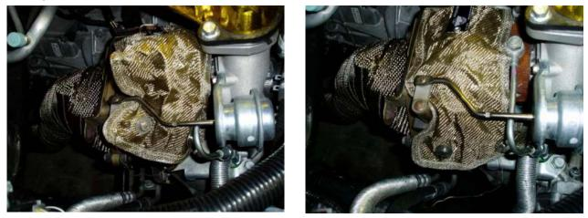
10.) Tie the stainless-steel wire around the rivets exactly the same way you did on the opposite end. Make sure that the blanket fits tightly over the turbocharger.
