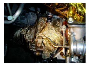
You may re-install your factory heat shield if you desire. Our Subaru turbo blankets can be used in conjunction with or without the factory heat shield.
