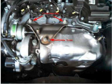
4.) After the mounting bracket has been removed you will remove the stock heat shield. Remove the three small 10mm nuts toward the top of the heat shield, as well as the two 10mm buts on the bottom. The two bottom nuts, toward the front of the engine, will require a standard 10mm wrench or a deep socket.
