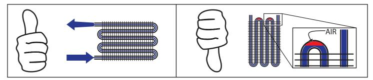
"Tank" type coolers (like a radiator) are a little more forgiving and offer one additional mounting option. The first option is the same as is recommended for the "tube" type cooler - the main tubes, or tanks, should run horizontally with the fluid entering the lower tank and exiting the top. The alternative is to mount the cooler so that the ports are pointed up. Since all the cooling rows are tied together at each tank, air should be able to exit the cooler using either mounting method.
