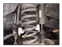
**STEP 7:** CAREFULLY lower front axle, then remove OE coil springs.
