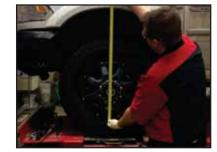
**STEP 2:** Position vehicle on a stable, flat surface or automotive lift. Suspend front wheels, lifting by the frame. Secure with jack stands & wheel chocks. Be sure engine is turned OFF and vehicle is in PARK.
