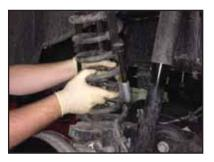
**STEP 8:** Remove OE rubber upper coil spring insulator, and save for reinstallation in step 10.
