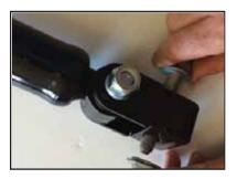
**STEP 10:** Install new adjustable upper lift kit in it lowest adjustment height, along with the OE coil spring and rubber upper coil spring insulator (removed in Step 8).
