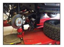
**STEP 4:** Unclip lower ABS, vacuum & brake line brackets to  $\varsigma$ »–"  $\P$ » $\varsigma$ %.
