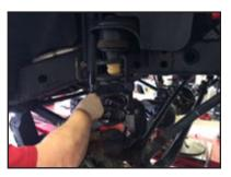
**STEP 7:** Remove lower front shock hardware and retain for reinstallation in step 14.
