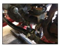
**STEP 6:** Install coil spring clamps, if available. This will simplify removal & rein-stallation of coil springs.
