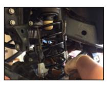
**STEP 9:** Determine your desired front lift height from 1.5" to 3.0", combining spacers as required. The largest spacer w/ logo should always be the **LOW-EST** spacer installed. The actual lift value will be the same as the thickness of the combined spacers.
