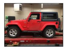
**STEP 2:** Position vehicle on a stable, fl t surface or automotive lift. Suspend front wheels, lifting by the frame. Secure with jack stands & wheel chocks. Be sure engine is turned OFF and vehicle is in PARK.
