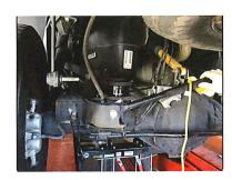
**STEP 11:** Reinstall OE coil springs into their original position.
