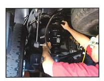
**STEP 12:** Reconnect lower shock mounts on each side of vehicle, as shown.
