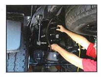
**STEP 6:** Remove rubber lower coil spring insulators.
