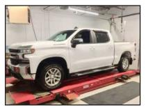
**STEP 2:** On a flat, level surface, MEASURE preinstallation ride height, FRONT & REAR, and write down measurements. Front (L)\_\_\_\_\_\_ Front (R)\_\_\_\_\_\_ Rear (L)\_\_\_\_\_ Rear (R)\_\_\_\_\_\_ Rear (R)\_R RAAR (R)\_
