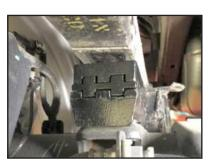
**STEP 9:** Slowly lower vehicle making sure the alignment pin lines up with alignment hole on block. Tighten new ubolts evenly in a crisscross pattern.
