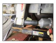
**STEP 11:** Progressively torque Ubolt nuts in a crisscross pattern to Factory specs.
