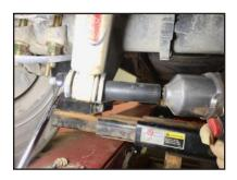
**STEP 12:** Progressively torque Ubolt nuts in a crisscross pattern to Factory specs.
