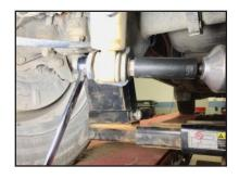
**STEP 5:** Remove the four U-bolt nuts and washers on each side of the vehicle, and remove lower U-bolt axle brackets.
