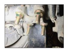
**STEP 11:** Install shock bolt and nut. Torque to manufacturer's specifications.
