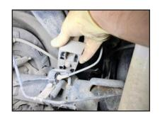
**STEP 7:** Install desired amount of lift. Make sure alignment pins line up with spring and axle. Make sure **FRONT** marking on block is facing **FRONT** of vehicle. Utilize lower portion of block to get 1.0" rear lift as shown here.
