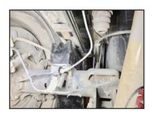
**STEP 8:** Utilize two lower blocks together to get 1.5" rear lift as shown here.
