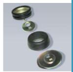
T. Offset Strut Tops For popular Volkswagen applications. Replaces the OEM upper bearing plate for camber and caster adjustment of +/- 1.0 degree.
