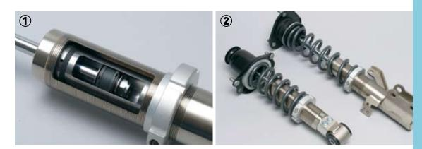
THE ORIGINAL TAKE-APART Coil-over System for Sport-Compact cars. This system has been refined over thousands of street and racing miles. Take PROGRESS Technology to the track and build a winner! PROGRESS Competition Series systems have been developed specifically for dual-purpose autocross, track day and drag race applications.
