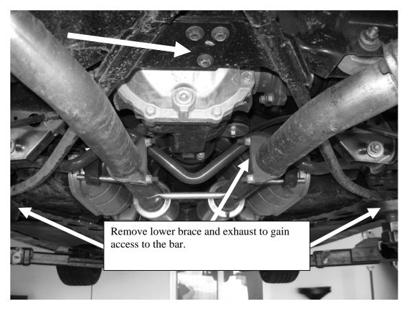
2. Remove rear wheels and tires. Remove the rear lower sub-frame brace and one side of the exhaust to gain access to the rear bar.
