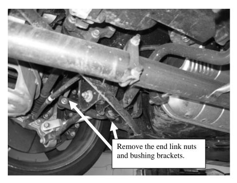
3. Remove the nuts that hold the end links to the bar. Next, remove the factory bushings and brackets, keeping the hardware. Remove the bar from the vehicle.
