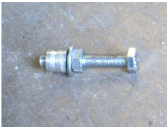
FIG 1 Nutsert shown ready to install
