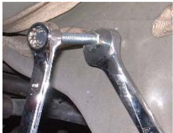
FIG 2 Hold bolt head and turn nut until tight
