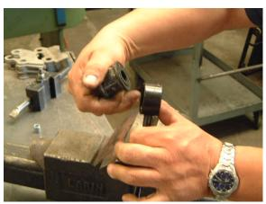
4. Next, remove the bushing from the lower eye in the factory link. Using a screwdriver pry the bushing out of the bore.
