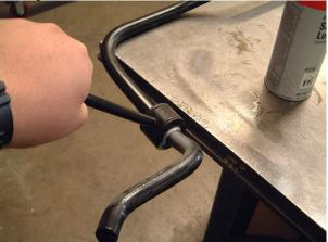
3. Remove the link and bushing from the factory sway bar; use a spray silicone to help slide them off the factory bar.
