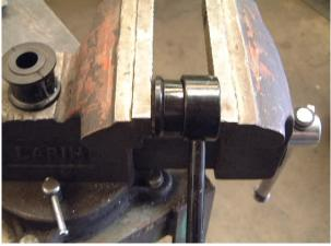
5. Coat the outside of the new bushing with silicone spray. Using a vice or press, install bushing into link.
