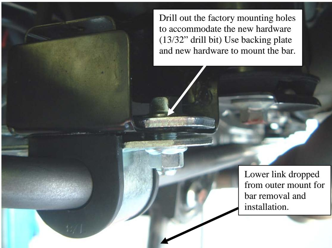
3. Drill out the existing holes for the bushing brackets using a 13/32" drill or uni-bit so that the supplied hardware can be installed. Place backing plate inside the factory mounting point so that a sandwich effect is made and a stronger mounting point is achieved. Install the M10 bolts from the top of the backing plate down thru the drilled out holes.
