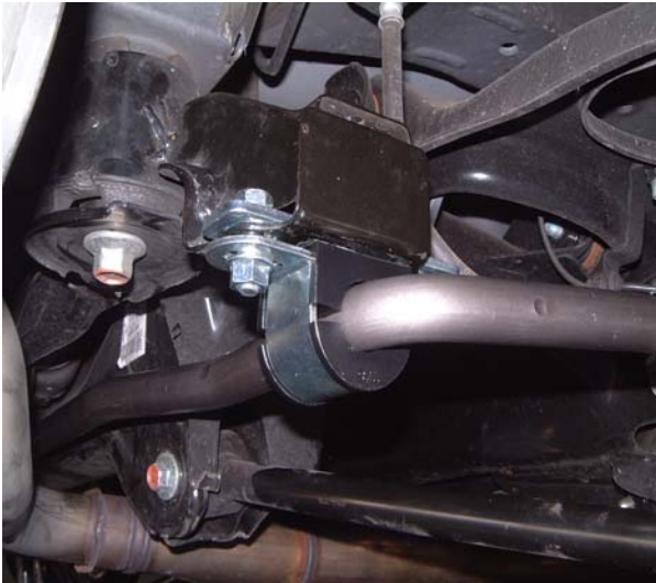
Center the bar and bracket on the mount before tightening.
