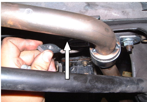
Use a spacer under the rear side of the bushing bracket, between the bracket and the chassis.
