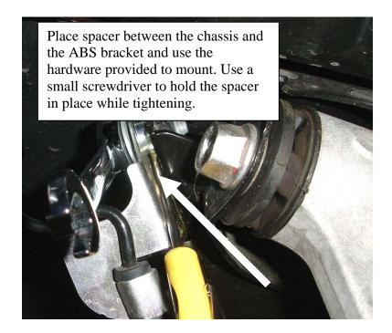
3. Attach end link, radiator mounts and ABS wires **with spacer behind it**. Torque all fasteners to factory specifications. Attach splash tray then install wheels and tires. Lower the front of car onto ground, and roll car back and forth to settle suspension.
