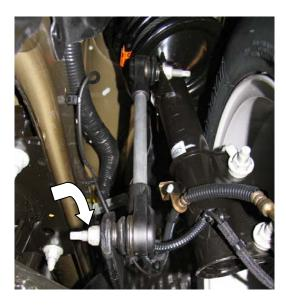
2. Locate and remove the nuts that attach the ends of the OEM anti-sway bar to the end links. It is not necessary to remove the end links from the strut. Retain these nuts for re-installation. Remove the bolts that attach the bar mounting brackets to the frame, and remove the OEM anti-sway bar from the vehicle.
