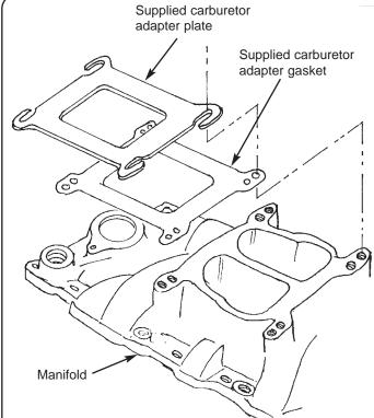
**Figure 2** - Manifolds 52000/52001, 52006/52007, 52008/52009, and 53000/53001 are designed to accept the stock style spread bore carburetor. To use a square bore carb, you must utilize the supplied carb adapter plate and gasket or air leakage will occur at the base of the carburetor.
