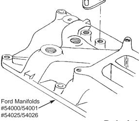
Figure 3 - In order to use both the early or late style stock Ford throttle bracket with our manifold, you will need to utilize the supplied adapter bracket as shown in the drawing at left.
