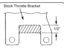
Figure 1 - Remove material from shaded area to provide clearance for throttle bracket or kick-down bracket, or use an Edelbrock #8036 bracket.
