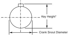
This is where you measure the installed key height and crank snout diameter. Note: Measure the SB and BB Chevv snout diameters halfway back from end of crank.
