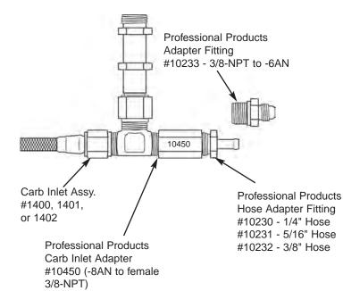
All Professional Products Carb Inlet Kits come with a -8AN male fitting for the fuel inlet line hookup. If you need to use -6AN or a slip-on hose fitting, use our #10450 Carb Inlet Adapter in conjunction with your choice of any of our three hose fittings or our -6AN fitting. See illustration at above.
