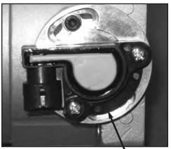
Grind away a portion of the plastic flange of the T.P.S. for access to adapter plate screw.
