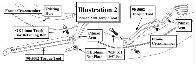
to be turned in order for the hole in the torque tool and the frame crossmember to line up. Once the bolts are tightened the torque tool will align it's self properly.
