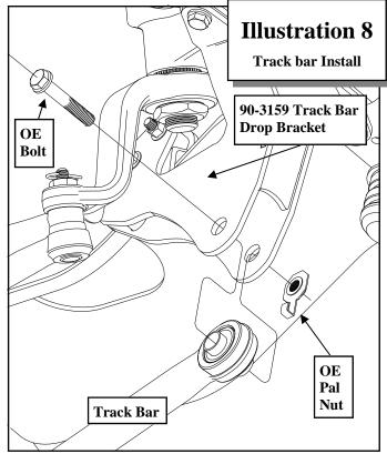
NOTE: You may find that having someone inside the vehicle and moving the steering wheel from side to side will aid in the alignment of the track rod. <u>DO NOT</u> start the engine for this! You only have to move it enough to line the holes up on the track bar mount.
