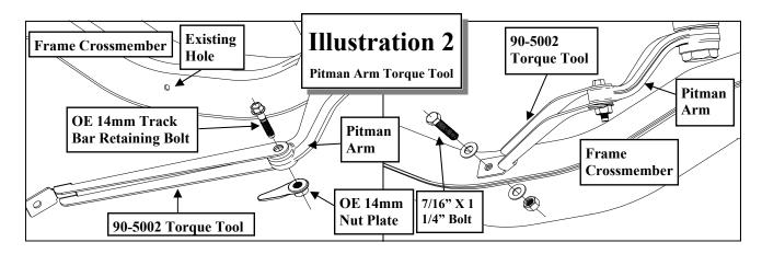
using the supplied 7/16" X 1 1/4" bolt and hardware. See Illustration 2.
