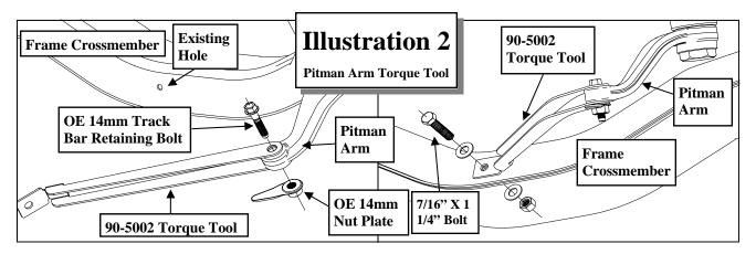
NOTE: The steering wheel may need to be turned in order for the hole in the torque tool and the frame crossmember to line up. Once the bolts are tightened the torque tool will align it's self properly.
