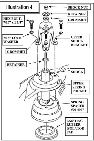
holes aligned, re-install the three **7/16**" **x 1-1/4**" hex bolts and lock washers through the bracket, spring pocket and into the threaded holes in the spring spacer. Torque to 35 ft./ lbs.
